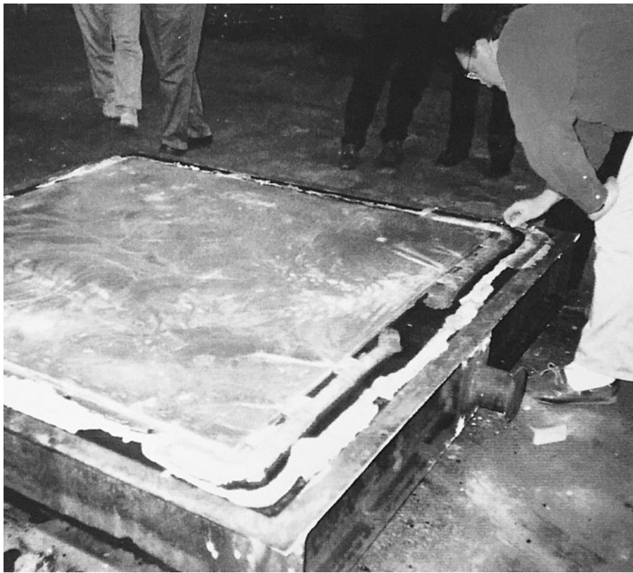
A cast-aluminum panel is inspected within its mold.
