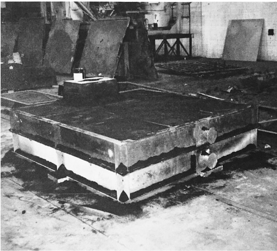
A 5'6" x 5'6" sand-cast mold waits to be filled.
