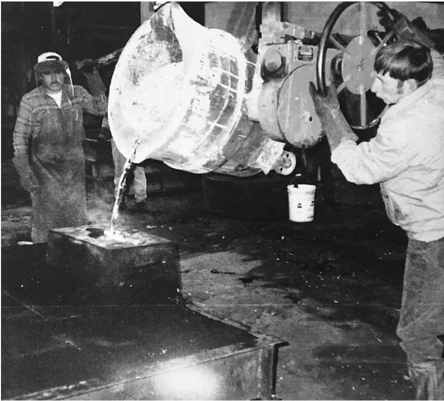
Molten aluminum is poured into a sand-cast mold.
